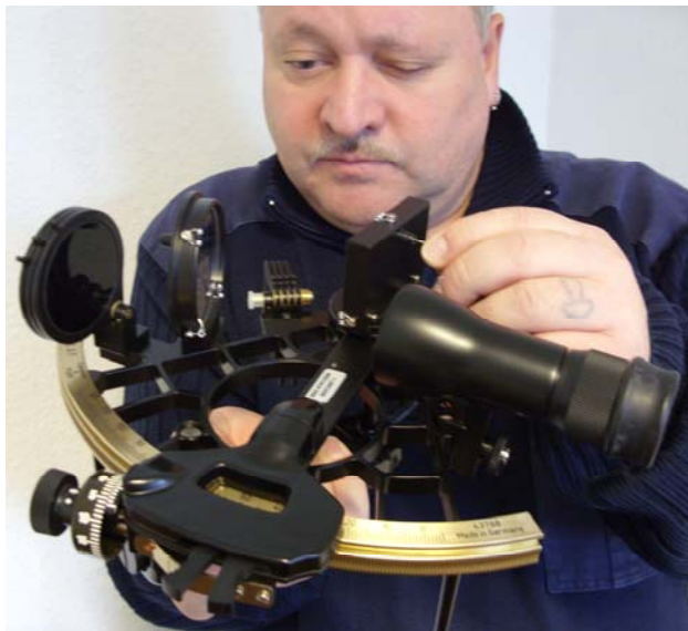
Take the sextant this way to identify and correct tilt error of index mirror
