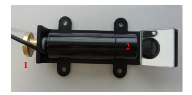
To adjust camera loosen arrest knob (1). Rotate camera until image is centered. Fix camera in that position with arrest knob. After that focus camera by turning the camera lens (2).
