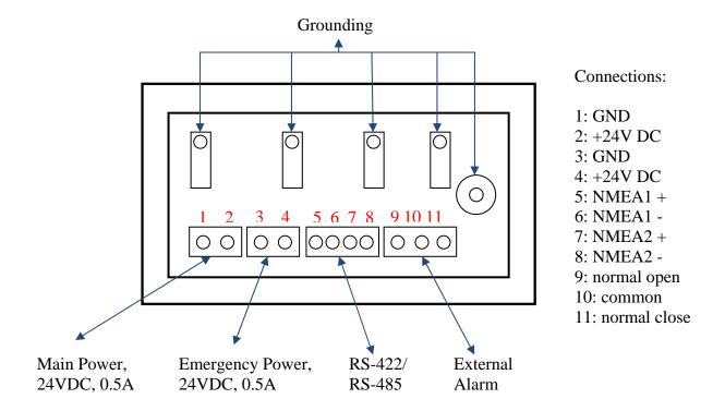
Cables have to been screwed to the terminals.
