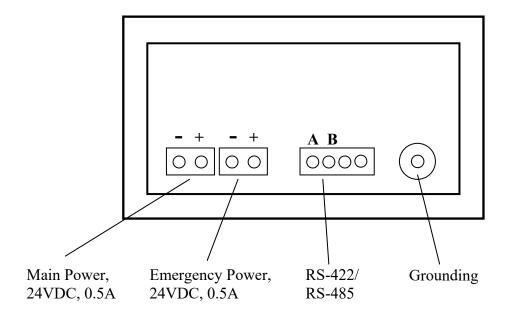
Cables have to been screwed to the removable terminals.
