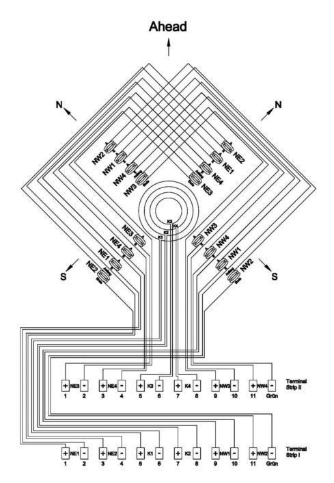
**Connection of Electro Compensation Coils**
